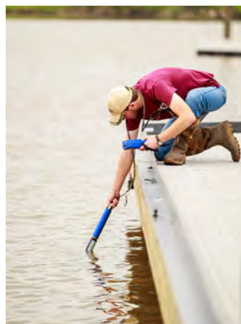
Ambient Water Quality Testing (Source Ed Rhodes, Texas Water Resources Institute)
